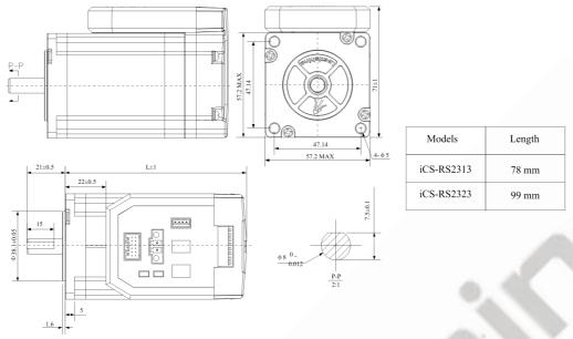
Figure 1: Mechanical specifications
