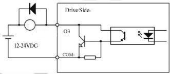
Figure 3.4: Output Interface Wiring
