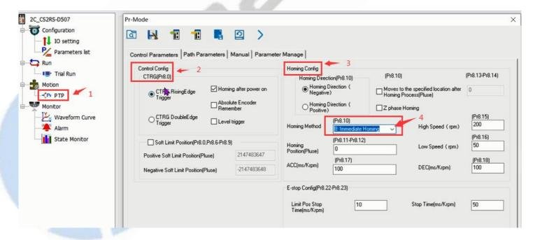
(2) This window is the PR path parameter setting, including operation mode, target position, speed value, etc. Double click to modify parameters.
