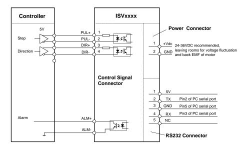
Connect iSV-Bxxx to controller of differential output
