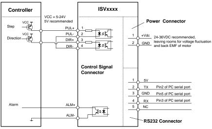
Connect iSV-Bxxx to controller of sourcing output
