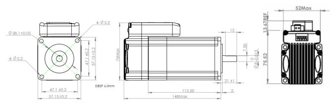
Mechanical Specification of iSV-B23180T-D4
