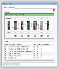
When using fieldbus axes connected to a MC4N, MC664 or MC464, *Motion* Perfect v4 can access and display bus status and node specific information.
