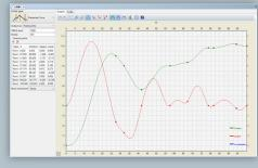
Define and generate cam tables using this interactive graphical cam designer. Commonly used cam shapes are pre-built into the CAM library software.
