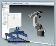
The 3D Visualization tool, available in *Motion* Perfect v4, enables simulation of Machine Motion, using an externally generated 3D model which can be synchronized with the motion program. This tool can simulate realistic movement sequences on a PC in real time.
