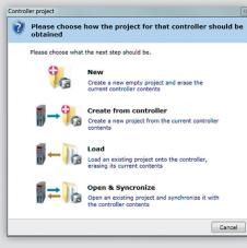
The multi-tasking capability of *Motion Coordinators* means there will be a number of different program files to make an application. In order to keep track of these multiple files and their associated data, a major component of the *Motion* Perfect v4 environment is the project manager.
