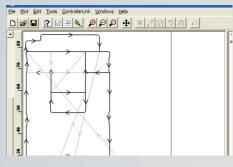
CAD2Motion is a program designed to allow users to translate CAD generated two dimensional motion paths into TrioBASIC programs.
