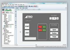
Trio's unique UNIPLAY HMI system keeps all the application programming in one place. No need for a separate HMI programming tool. *Motion* Perfect v4 comes with a built in visual editor for the Trio UNIPLAY HMIs.
