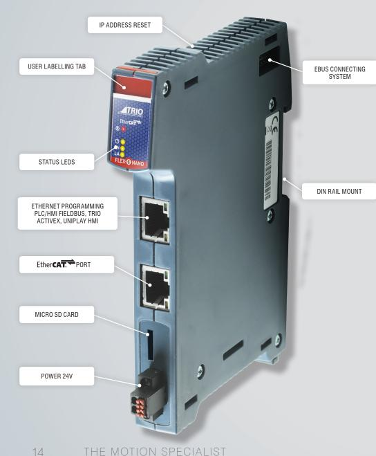
The Flex-6 Nano is a compact, integrated EtherCAT solution offering up to 64 Axes of motion. The on-board memory can be boosted to 32 GByte with the addition a micro SD card.
