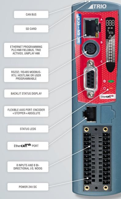
The MC6N is a high performance *Motion Coordinator* which is able to run up to 64 remote servo and stepper drives via the EtherCAT real time bus. It runs a 1GHz Dual Core processor making it ideal for high axis count machines or robotic applications.
