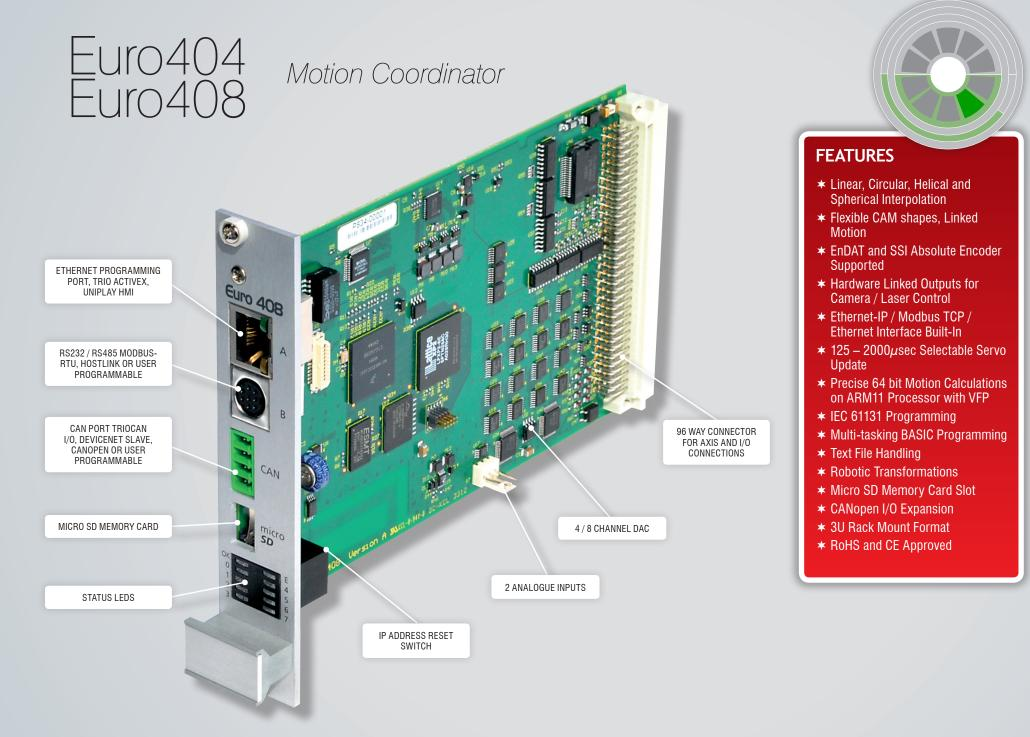
The Euro404 and Euro408 *Motion Coordinators* are designed to provide a powerful yet cost effective control solution for OEM machine builders that are prepared mount the unit and provide the power supplies required.
