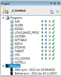
One of the keys to using *Motion* Perfect v4 is its concept of a "Project". The project aids the application design and development process, by providing a copy of the multiple controller programs, parameters and data required for a single motion application, all stored in one folder.
