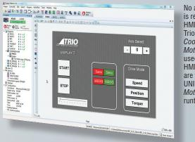
No additional software is required; UNIPLAY HMI's work with the Trio MC4+ Motion Coordinator range. Motion Perfect v4 is used to create operator HMI screens which are transferred to the UNIPLAY HMI by the Motion Coordinator at runtime.
