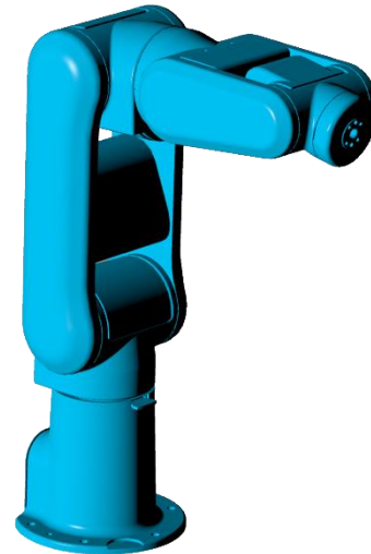
Figure 9-2: C := 1, Wrist flip, elbow above, base forward.
