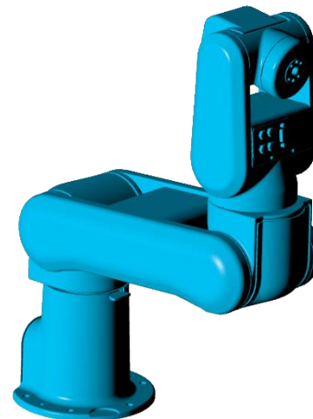
Figure 9-4: C := 3, Wrist flip, elbow below, base forward.
