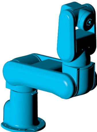
Figure 9-3: C := 2, Wrist no flip, elbow below, base forward.
