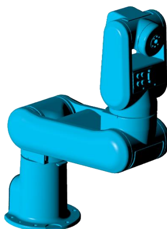
Figure 9-6: C := 5, Wrist flip, elbow below, base backward.
