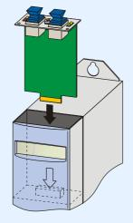
5. Secure the metal plate on the PCB with the included screws:
