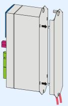
3. Press the device down on the guides:
