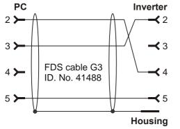
Fig. 7-1 Serial connection to communication between inverter and PC
