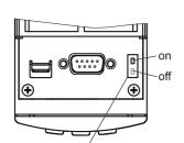
internal terminating resistance 120  $\boldsymbol{\Omega}$  can be activated
