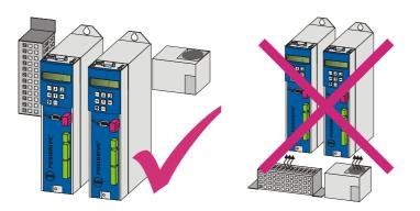
• To ensure there is sufficient air circulation in the control cabinet, observe the minimum clearances.
