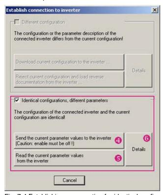
Fig. 7-4 Establishing a connection for identical configurations
