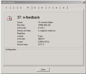
Fig. 8-1 View of the fault memory
