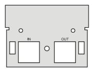
the following cover plate, which is included in the accessories, is required for installing the PN 5000:
