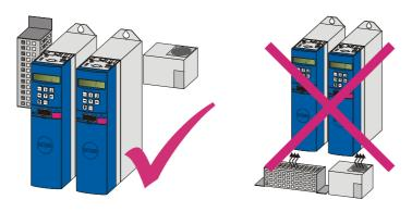
• To ensure there is sufficient air circulation in the control cabinet, observe the minimum clearances.
