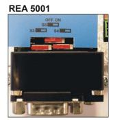
Please note that the switches are installed in different positions on the REA 5001 and XEA 5001 accessories. Identification of the switches and assignment of the switch positions to the function (switched on/switched off terminal resistance) are shown on the PCB cover.
