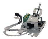
Accessory part for direct control of up to two motor holding brakes (24 V/DC). Attachable on the basic housing. Including connection cable for basic device and shield connection terminal for power cable cross-sections of 1 to 10 mm<sup>2</sup>.
