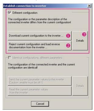
Fig. 7-3 Establishing connection with different configurations
