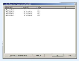
In the first column of this dialog screen, you can select the inverters which are connected to the PC. The possible targets in your project are shown in the second column.
