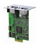
Accessory part for connecting EtherCAT (CANopen over EtherCAT).
