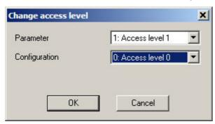
Fig. 6-2 Setting the access levels
