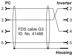
Fig. 7-1 Serial connection to communication between inverter and PC
