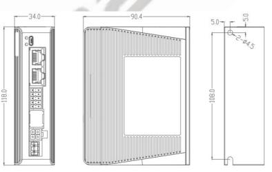
Figure 2.1: CS3E-E-522E/556E/870E Mechanical Drawing
