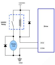
Figure 3.6: Brake output connection
