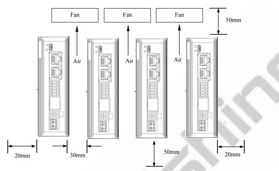
Figure 2.2: CS3E-E series installation drawing
