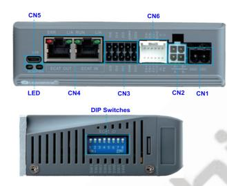
Figure 3.2: CS3E-E series connectors
