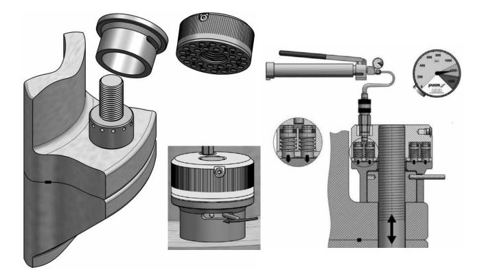
Hydromechanical Preload Device I HVV-A Series Axial Operation - from above
