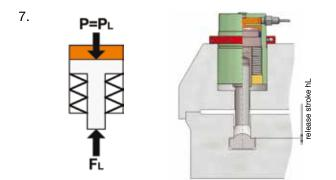
load with release pressure  $\mathsf{P}_{\scriptscriptstyle L}$  , disk spring package is compressed further
