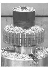
✓ with threaded pin ✓ function as power clamping screw ✓ centered operation ✓ compact design
