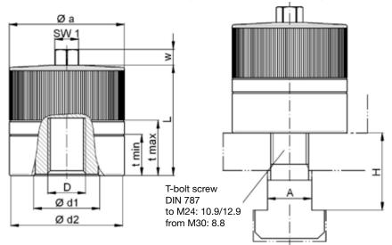
material: heat treated steel - nitro carburized cover plate: high tensile aluminum
