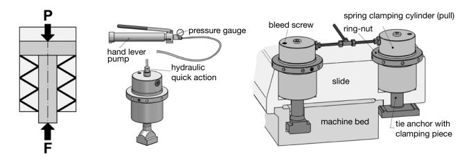
Note: If automatic clamping operation is not required, the temporary, manual hydraulic connection to a manually operated piston pump with a pressure gauge provides a cost effective alternative (see fig. at left).
