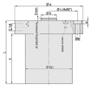
*material:* heat treated steel, burnished or nitro carburized
