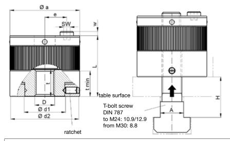
*material:* heat treated steel - nitro carburized
