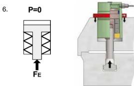
release hydraulic pressure - P = 0 bar - clamping force of disk spring package =  $F_{N}$
