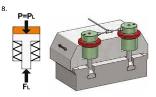
T-bolt screw and tensioning bolt are in release position. Slide can be moved axially
