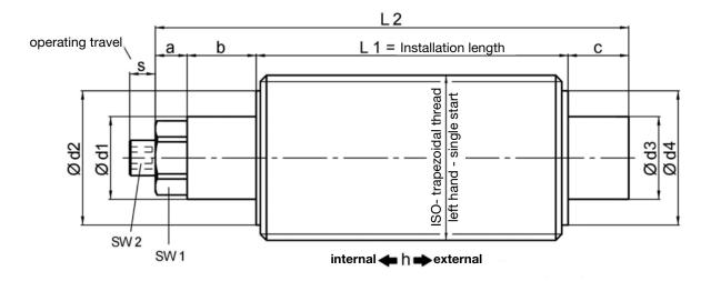
*material:* heat treated steel - nitro carburized
