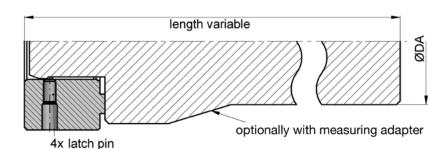
The inner diameter of the ring load cells is primed for the insertion of measuring adapter pieces using four ball latch pins. Customized adapter types are available on request (see example of use).
