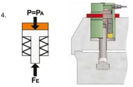
load cylinder with adjusting pressure  $P_A$  - disk spring package is compressed - T-bolt screw is released by stroke of pressure piston
