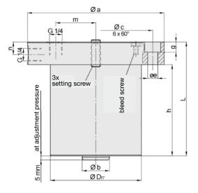
material: heat treated steel, burnished or nitro carburized
