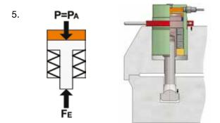
turn ring nut until ring nut and tensioning bolt are at mechanical stop - lock ring nut with screw
