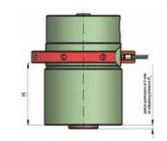
adjust ring nut to mounting position (M) and lock
