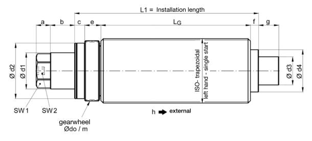
material: heat treated steel nitro carburized
