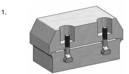
T-bolt screw or tension bolt installation (consider twist lock)
