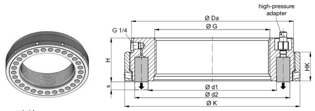
*material:* heat treated steel - nitro carburized
