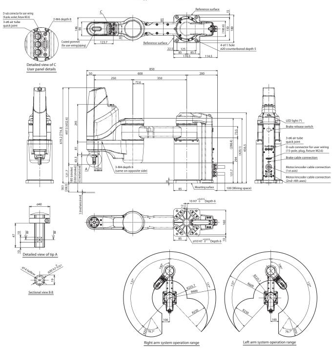
$(*) \ \ \text{To operate the LED, wire a controller output to apply 24VDC to the LED terminal of the user wiring.}$
