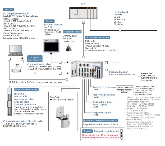
(Note) When connecting an actuator with brake, the brake power supply +24V is required for the controller.
