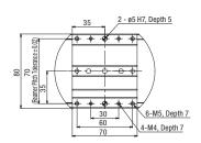
Detailed Diagram U (Detail of Y-axis Slider)
