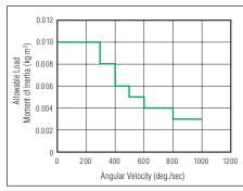
Allowable load moment of inertia, angular velocity, angular acceleration and deceleration (R)
