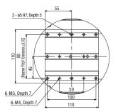
Detailed Diagram S (Detail of X-axis Slider)
