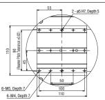
Detailed Diagram S (Detail of X-axis Slider)
