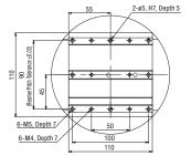
Detailed Diagram S (Detail of X-axis Slider)
