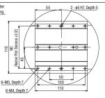
Detailed Diagram S (Detail of X-axis Slider)
