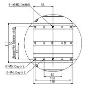
Detailed Diagram S (Detail of X-axis Slider)
