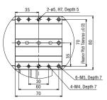
Detailed Diagram U (Detail of Y-axis Slider)
