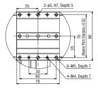
Detailed Diagram U (Detail of Y-axis Slider)
