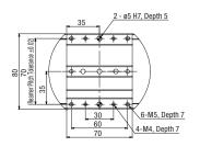
Detailed Diagram U (Detail of Y-axis Slider)
