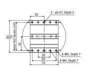
Detailed Diagram U (Detail of Y-axis Slider)
