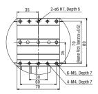
Detailed Diagram U (Detail of Y-axis Slider)
