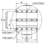
Detailed Diagram S (Detail of X-axis Slider)
