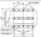
Detailed Diagram S (Detail of X-axis Slider)
