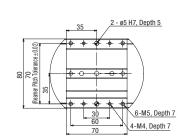
Detailed Diagram U (Detail of Y-axis Slider)
