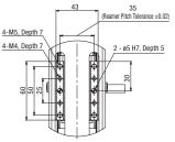
Detailed Diagram U (Detail of Z-axis Slider)
