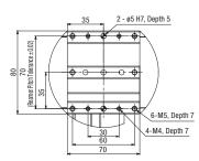
Detailed Diagram U (Detail of Y-axis Slider)
