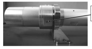
2 affixing bolts on the motor-end cap (right and left) (hexagon socket head setscrews)
