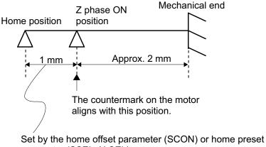
parameter (SSEL, X-SEL). (The above value indicates the factory setting.)
