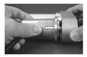
4) Install the replacement motor. Loosely tighten the motor-unit affixing bolts.
