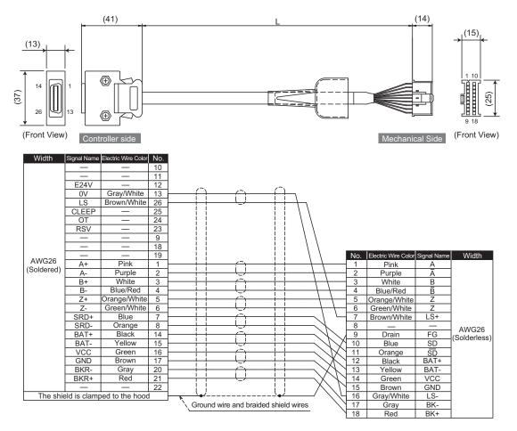
[Bending Radius] When used under moving condition : 58mm (Robot Cable) When used in fixed condition : 93mm (Standard Cable)
