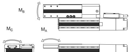
The point of action for the moment in directions Ma and Mb are as shown below.
