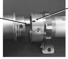
Apply a countermark at a position corresponding to the tab on the motor unit.
