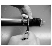
Tightening of rear metal fitting
