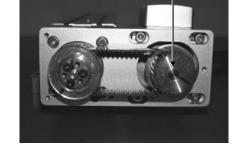
3) Remove the belt from the pulleys.
