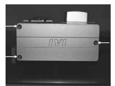
2) Loosen the four tension adjustment bolts to slacken the belt.
