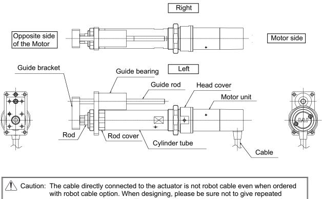
with robot cable option. When designing, please be sure not to give repeated bending loads to this cable. The robot cable is applicable only to the connecting cables.
