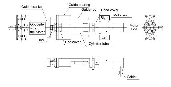
6. Motor Reversing Type: With Double Guides
