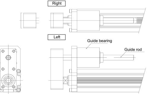
10. Motor Straight Type (Coupling Type): Double-guide Type
