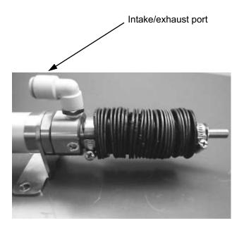
Install the air tube (outer diameter: 10 mm, inner diameter: 6.5 mm) on the intake/exhaust port and guide the air tube to a location where the external environment assures the tube will not come in contact with water.
