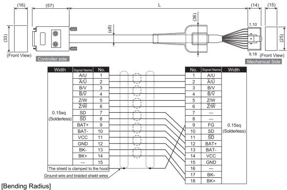
When used under moving condition : 90mm (Robot Cable) When used in fixed condition : 75mm (Standard Cable)
