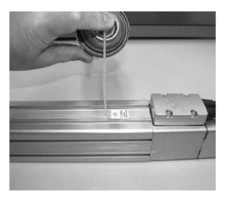
3) After grease has been applied, move the rod back and forth to let the grease spread evenly.
