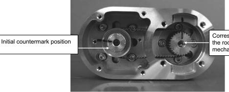
Corresponding to a position where the rod projects 2 mm from the mechanical end
