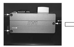
Loosen the four tension adjustment bolts to slacken the belt. (Allen wrench of 3 mm across flats) Check the rotating direction of the motor shaft.
