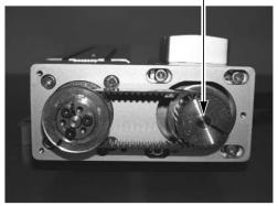
3) Remove the belt from the pulleys.
