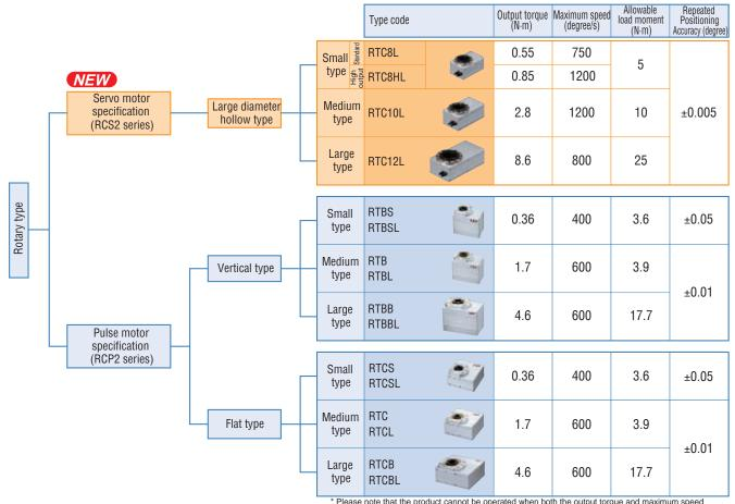
\* Please note that the product cannot be operated when both the output torque and maximum speed values are simultaneously at the settings given in the above table.
