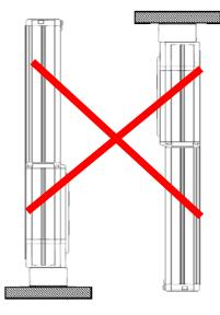
When using the product in horizontal or vertical orientation, have a support block to support the main body to avoid any external force to be applied on the body.
