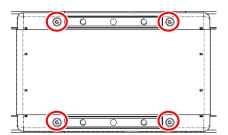
(3) Remove the two hex socket button head bolts on each of left and right sides with using a 2mm-sized (for WSA10C/10R) or 2.5mm-sized (for WSA12C/12R, WSA14C/14R and WSA16C/16R) hex wrench, and detach the retainer plate and the old stainless steel sheet.
