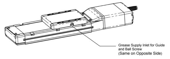
(Note) Prepare a grease gun suitable for the diameter of the grease nipples stated below.
