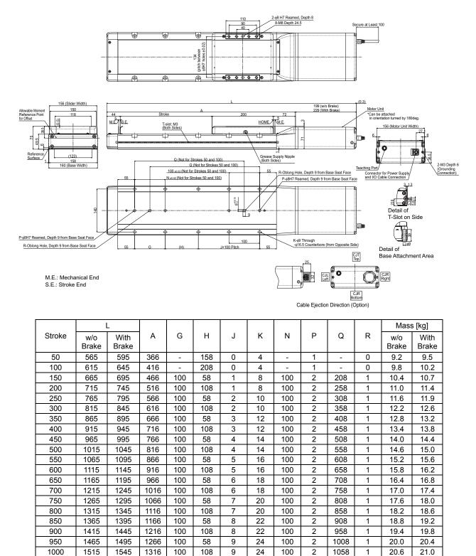
21.8 (Note) L dimensions described in the table are those with no cable ejection direction (option). For cable ejection direction types (option), the dimensions are longer in 25mm.
