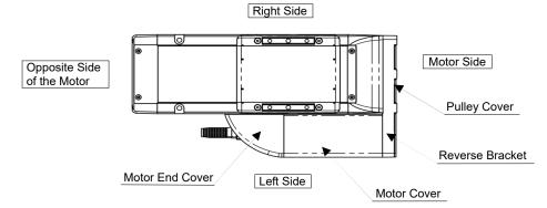
The direction of the motor is either left reversed: ML (shown in figure above), right reversed: MR.
