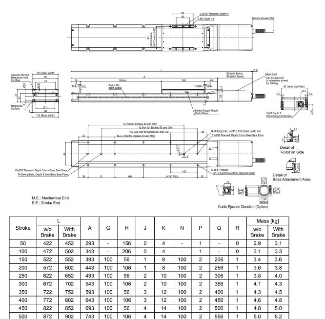
(Note) L dimensions described in the table are those with no cable ejection direction (option). For cable ejection direction types (option), the dimensions are longer in 25mm.
