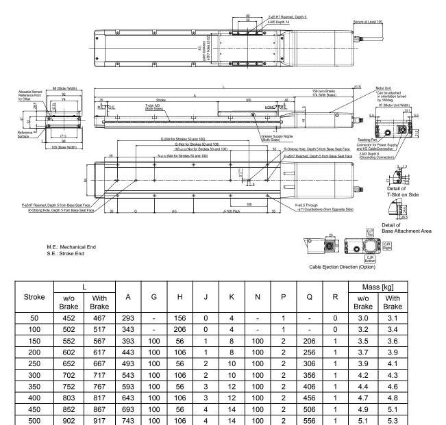
(Note) L dimensions described in the table are those with no cable ejection direction (option). For cable ejection direction types (option), the dimensions are longer in 25mm.
