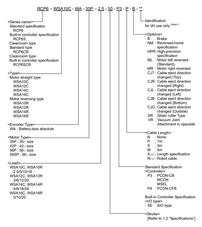
Note 1 Identification for IAI use only: It may be displayed for IAI use. It is not a code to show the model type. \* The slider roller type SR is an option for the standard type RCP6 and the controller built-in type RCP6S.
