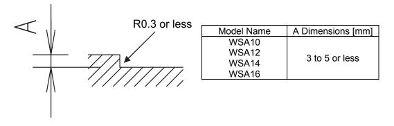
Caution: As there could be a case that the width dimension of the front bracket or rear bracket is wider than the datum surface dimension on the side, have them pushed towards the datum surface within the datum surface effective range. Having machining work to press the brackets towards the datum surface outside the datum surface effective range may cause interference to brackets and motors.
