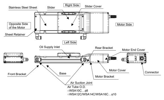
3.2 Built-in Controller Specification RCP6SCR-WSA10C、WSA12C、WSA14C、WSA16C
