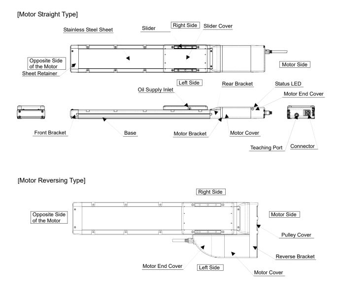
The direction of the motor is either left reversed: ML (shown in figure above), right reversed: MR.
