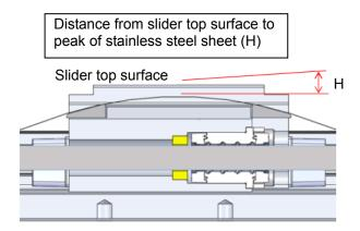
Distance between Peak of Stainless Steel Sheet and Slider Top Surface
