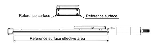
As shown in the figure above, the base side surface is the datum surface for the slider drive. Have this surface as the datum for installation when accuracy is required.
