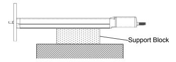
Operation of the actuator with attachment only on the front bracket applies the external force of the acceleration/deceleration multiplied by the weight of the actuator to the unit body. Control the acceleration/deceleration at 0.05G or less (for reference) when the actuator is moved with attachment only on the front bracket.
