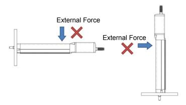
Prepare a support block as shown in the figure below for the horizontal installation of the unit with its stroke more than 150 even if there is no external force applied on the body. Even for those with the stroke less than 150, it is recommended to have a support block to avoid vibration being generated due to the operation condition or installation environment, which may cause an operation failure or parts malfunction.
