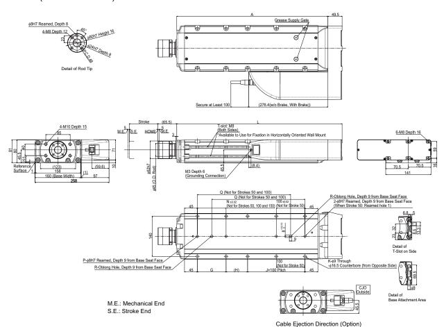
Mass [kg] Ρ Stroke L G Н Κ Ν Q R w/o With Brake Brake 326.5 13.1 13.3 376.5 14.2 14.4 426.5 15.3 15.6 16.5 16.7 476.5 526.5 17.6 17.9 576.5 18.7 19.0 626.5 19.9 20.1 676.5 21.0 21.3 22.2 22.4 726.5 776.5 23.3 23.5 24.5 24.7 826.5 876.5 25.6 25.8 27.0 926.5 26.7 976.5 27.9 28.1 29.0 29.3 1026.5 1076.5 30.1 30.4
