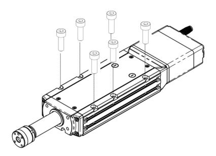
Apply the socket head cap screw indicated in the table below suitable for the platform material.
