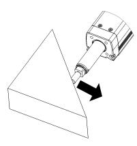
Be careful on the direction of the reaction force against the pressing. operation.
