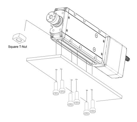
On the T-slot, square T-nuts specified in JIS B 1163 are available to use.
