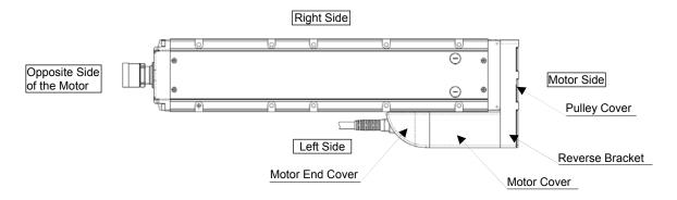
The direction of the motor is either left reversed: ML (shown in figure above) or right reversed: MR.
