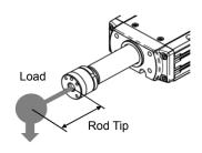
[Rod Tip Allowable Torque]
