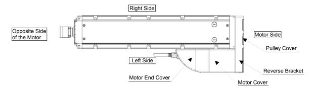
The direction of the motor is either left reversed: ML (shown in figure above) or right reversed: MR.
