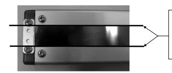
There are two grooves for stainless steel sheet attachment guides. Align so that the stainless steel sheet is positioned at the center between the two grooves. Attach the stainless steel sheet so that it is not bent.
