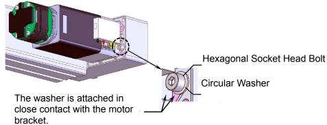
4) Loosen the bolts (where marked with a circle; two bolts for SA4R and SA6R, four bolts for SA7R, and SA8R) holding the motor with a 2.5mm-sized (SA4R) or 3mm-sized (SA6R/SA7R/SA8R) hexagonal wrench. Replace the belt if it is necessary.
