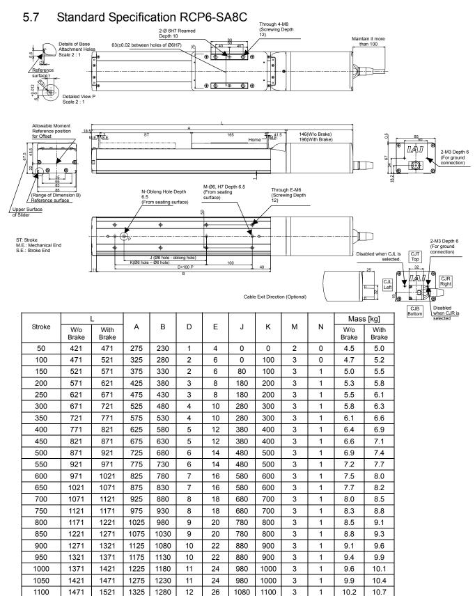
(Note) L dimensions described in the table are those with no cable exit direction (option). For cable exit direction types (option), the dimensions are longer in 25mm.
