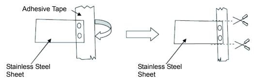
Attach adhesive tape so that it wraps around the end side of the stainless steel sheet. At that time, arrange it so that about 3mm of the end of the tape projects from the stainless steel sheet. Cut any tape excess.
