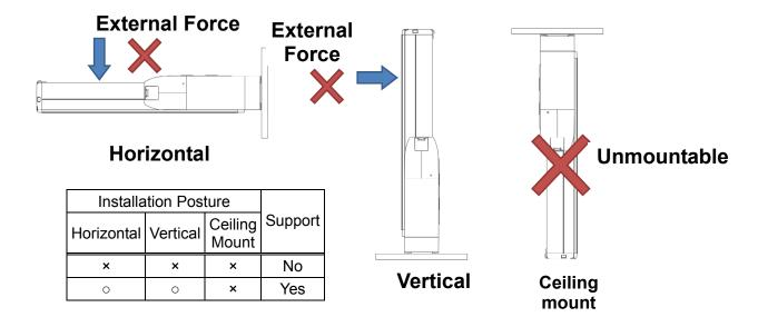
When using the product in horizontal or vertical orientation, have a support block to support the main body to avoid any external force to be applied on the body.
