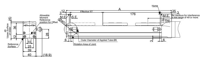
Effective ST: Effective Stroke M.E.: Mechanical End S.E.: Stroke End
