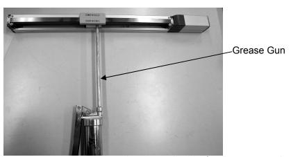
(Note)Make sure to use a grease gun that is applicable for the grease nipple inlet diameter shown below.
