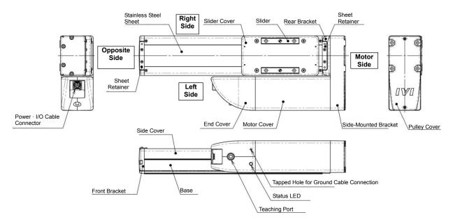
The direction of the motor is either left side-mounted: ML (shown in figure above), right side-mounted: MR.
