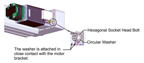
Loosen the bolts (where marked with a circle; two bolts for SA4R and SA6R, four bolts for SA7R, and SA8R) holding the motor with a 2.5mm-sized (SA4R) or 3mm-sized (SA6R/SA7R/SA8R) hexagonal wrench. Replace the belt if it is necessary.
