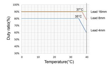
Duty ratio is an operating rate, which indicates the time that the actuator is running in one cycle by percentage.
