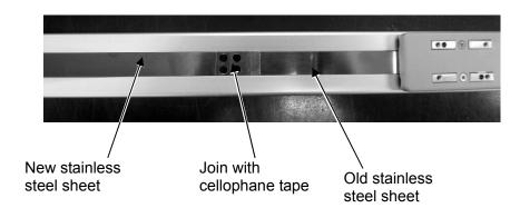
4) Pull the old stainless steel sheet so the new one goes through below the slider. Pull it till the new stainless steel sheet comes to the edge of the actuator.
