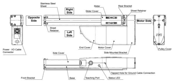
The direction of the motor is either left side-mounted: ML (shown in figure above), right side-mounted: MR.
