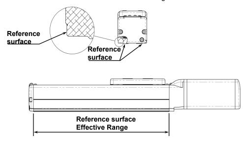
In the case that the accuracy is required, use the base side surface as reference surface for mounting, as this surface works as the reference surface for the running of the slider.
