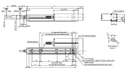
\* Dimension () is for brake-equipped
