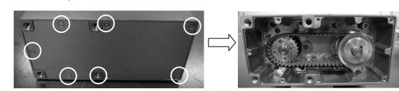
Loosen the four tension adjustment bolts (where marked with a circle) to loosen the belt. (Use a hexagon wrench with the distance to the opposite side of 5 mm (RA8R), 6 mm (RA10R))
