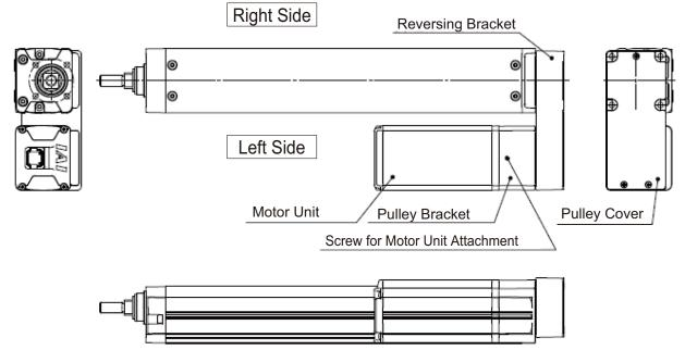
The direction of the motor is either left reversed: ML (shown in figure above, standard) or right reversed: MR (option).
