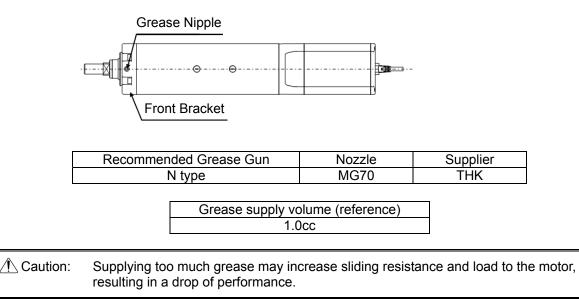
2) Slide the rod back and forth manually with hand or by the controller with JOG operation to spread out the grease evenly.
