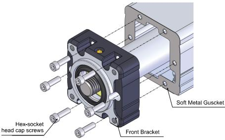
2) Attach the front bracket and tighten with bolts.
