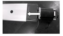
Insert the motor to the main body while the position of the key on the motor aligned to the key groove on the main body.
