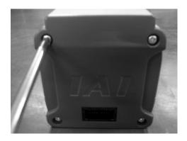
1) Remove the four screws holding the motor cover with using a Phillips screwdriver. The motor cover can be detached.
