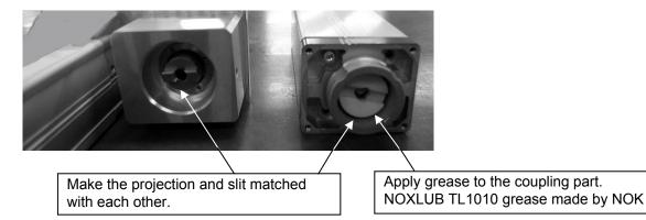
4) Attach the motor unit for replacement with the projection being matched with the slit.
