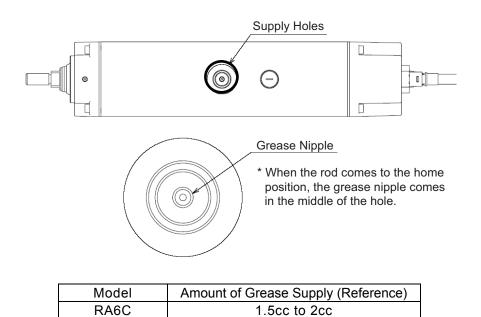
4) Slide the rod back and forth manually with hand or by the controller with JOG operation to spread out the grease evenly.
