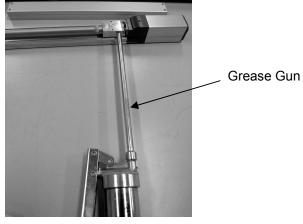
(Note) Make sure to use a grease gun that is applicable for the grease nipple inlet diameter shown below.
