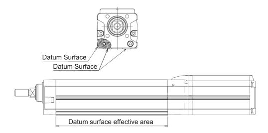
Follow the diagram below when installing the device using the reference surface.
