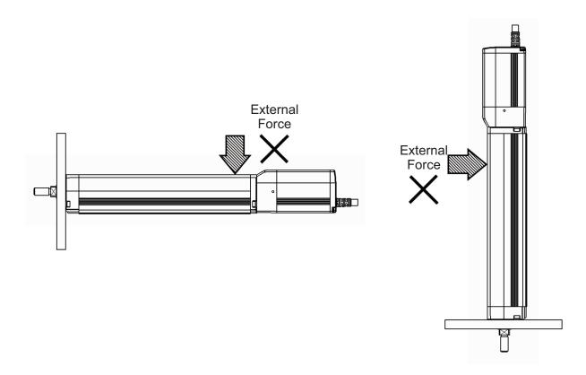
Prepare a support block as shown in the figure below for the horizontal installation of the unit with its stroke more than 150 even if there is no external force applied on the body. Even for those with the stroke less than 150, it is recommended to have a support block to avoid vibration being generated due to the operation condition or installation environment, which may cause an operation failure or parts malfunction.
