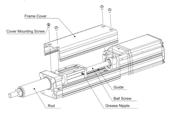
When affixing the frame cover, tighten the screws with the tightening torque described below.
