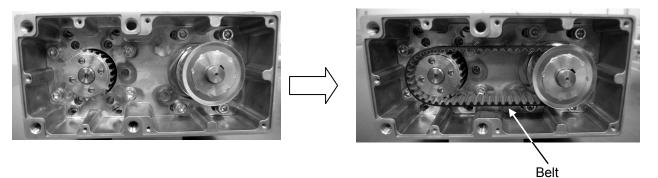
7) Put a strong string shaped in a loop (or a long tie-band) around the motor bracket, pull the string with a tension gauge to keep it in the specified tension force, and tighten the tension bolts (where marked with a circle) evenly.
