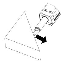
Be careful on the direction of the reaction force against the pressing
