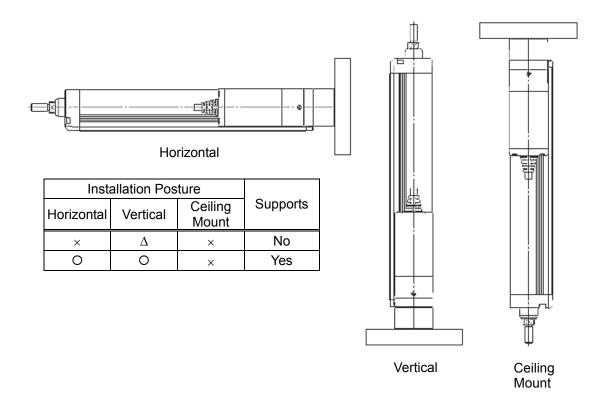
When using the unit in the horizontal or vertical orientation, have a pedestal to support the body to avoid external force being applied to the unit.
