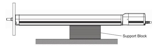
Operation of the actuator with attachment only on the front bracket applies the external force of the acceleration / deceleration multiplied by the weight of the actuator to the unit body. Control the acceleration / deceleration at 0.05 G or less (for reference) when the actuator of RA8 or RA10 is moved with attachment only on the front bracket.
