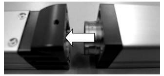
5) Tighten the fixing screw to affixing the motor unit to the actuator with 2mm-sized (RA4C, RA6C) or 2.5mm-sized (RA7C) hex wrench.
