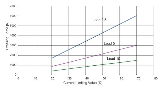
Due to the buckling load of the ball screw, there is a limitation in the pressing force for those with long stroke shown below.
