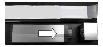
5) Tighten fixing screw to affixing the motor unit to the actuator with a 2mm-sized (RA4R, RA6R), 2.5mm-sized (RA7R) hex wrench.
