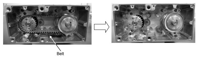
4) Pull out the four tension adjustment bolts and detach the motor unit.
