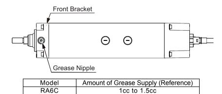
2) Slide the rod back and forth manually with hand or by the controller with JOG operation to spread out the grease evenly.
