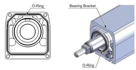
4) Attach the front bracket and tighten with bolts. At this time, pay attention not to pinch the O-rings in between.
