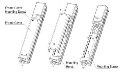
When affixing the frame cover, tighten the screws with the tightening torque described below.
