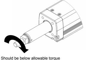
Should be below allowable load Do not attempt to apply impact load
