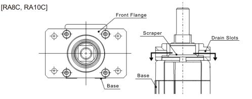
13. Dustproof/splash proof type RCP5W actuator is grease flows out gradually from the tip of the rod.
