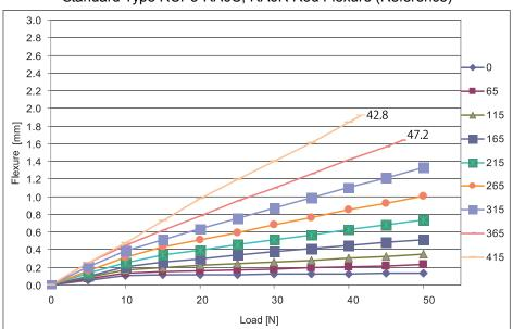
Standard Type RCP5-RA6C, RA6R Rod Flexure (Reference)
