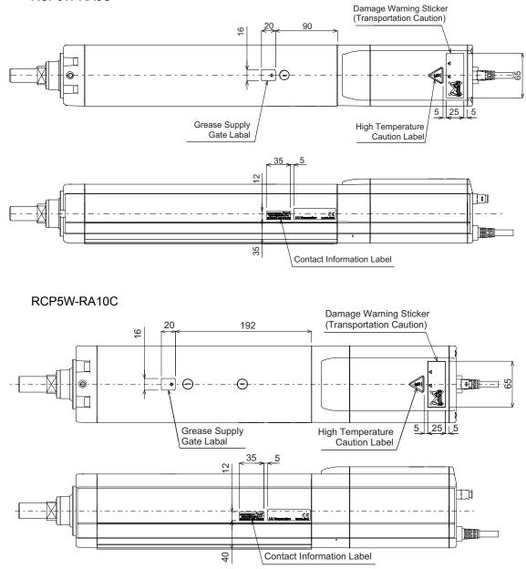
(Note) It is not necessary to attach the contact information label if the product is to be used besides japan. The contact information label shows the information of 24-hour contact in japan. The free-call number described on the label is only for japanese domestic use.
