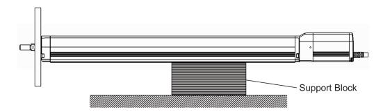
Operation of the actuator with attachment only on the front bracket and the front flange (option) applies the external force of the acceleration / deceleration multiplied by the weight of the actuator to the unit body.
