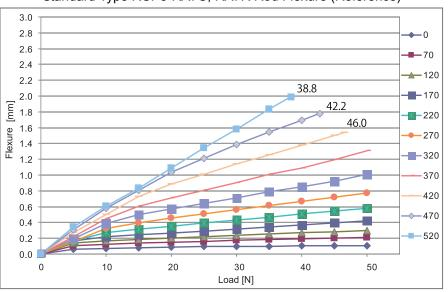
Standard Type RCP5-RA7C, RA7R Rod Flexure (Reference)
