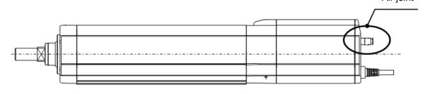
Caution: Do not attempt to suck in water through the air joint (air inlet/outlet port). Doing so may cause malfunction.
