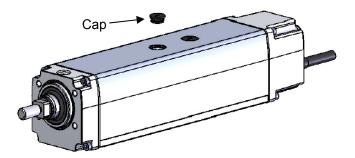
2) Move the rod to the end of the mechanical stopper on the home side.
