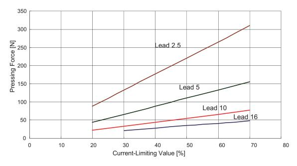
Caution: (1) The relation of the current limit and the pressing force is a reference when assuming the speed is 20mm/s.
