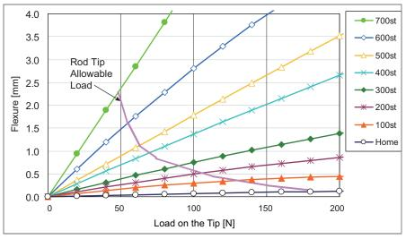
Standard Type RCP5-RA10C, RA10R Dustproof/Splash Proof Type RCP5W-RA10C Rod Flexure (Reference)
