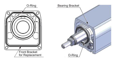
Attach the front bracket and tighten with bolts.
