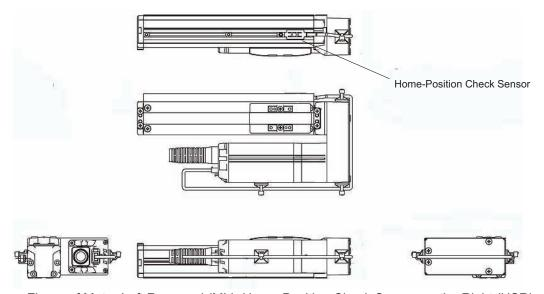
Figure of Motor Left Reversed (ML), Home-Position Check Sensor on the Right (HSR)
