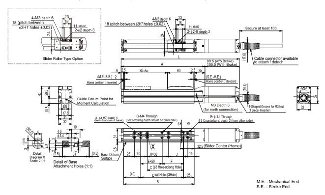
(Note) Be aware that the attachment holes available for installation of stroke 25 of SA3C are four places on the ends even through there are six attachment holes for attachment from the top.
