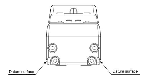
Because the side and bottom faces of the base provide reference surfaces for slider travel as shown in the above diagram, conduct installation based on the position of these sides when precision is required.
