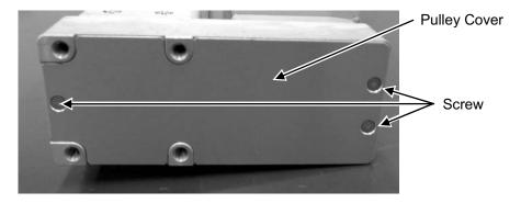
2) Loosen the four screws holding the pulley on the motor side with a 2.5mm-sized (SA3R/SA5R/SA6R) or 3mm-sized (SA7R) hex wrench. If the belt is required to be replaced, replace it.
