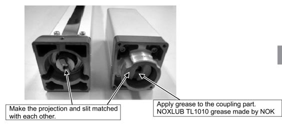
4) Attach the motor unit for replacement with the projection being matched with the slit.
