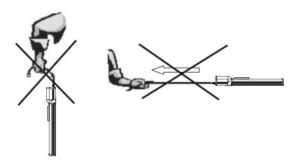
When transporting the unassembled actuator, pay attention to the items specified below. When unpacking the actuator and handling it thereafter, always hold it by the base. Never hold an actuator by the stainless sheet.
