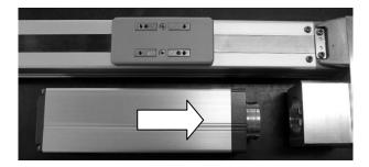
5) Tighten the fixing screw to affixing the motor unit to the actuator with 2mm hex wrench.
