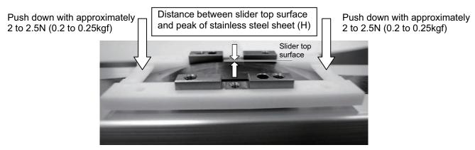
Distance between Peak of Stainless Steel Sheet and Slider Top Surface
