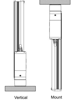
When using the unit in the horizontal or vertical orientation, have a pedestal to support the body to avoid external force being applied to the unit.
