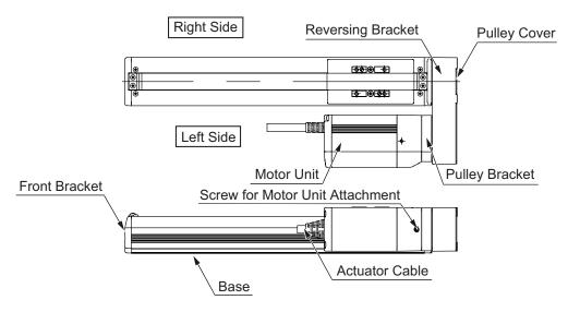
The direction of the motor is either left reversed: ML (shown in figure above) or right reversed: MR.
