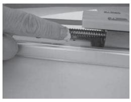
Move the slider back and forth in the stroke range after supplying grease so it spreads out evenly in the area.
