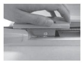
Caution: Supplying too much grease may increase sliding resistance and load to the motor, resulting in a drop of performance.
