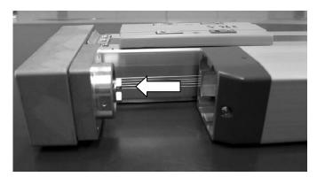
5) Tighten the fixing screw to affixing the motor unit to the actuator with 2.5mm hex wrench.
