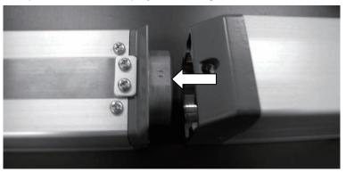
5) Tighten the fixing screw to affixing the motor unit to the actuator with 2.5mm hex wrench.
