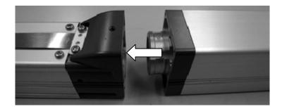
5) Tighten the fixing screw to affixing the motor unit to the actuator with 2mm hex wrench.
