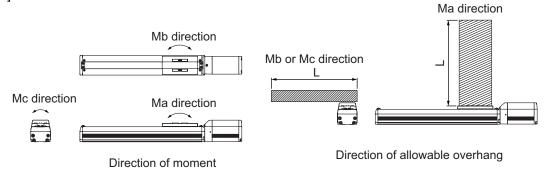
For the calculation of Ma and Mc moments, consider the position indicated with an arrow as the datum point.
