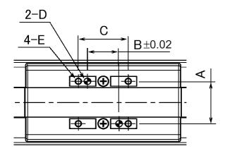
Reamed Hole Pitch Tolerance: ±0.02
