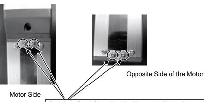
Stainless Steel Sheet Holder Plate and Fixing Screws Tighten on the motor side properly and leave the other side loose.
