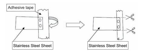
Attach adhesive tape so that it wraps around the end side of the stainless steel sheet. At that time, arrange it so that about 3mm of the end of the tape projects from the stainless steel sheet. Cut any tape excess.
