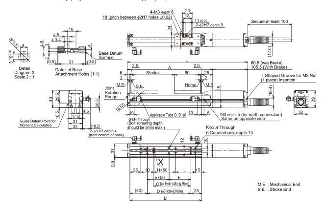
(Note) Be aware that the attachment holes available for installation of stroke 25 of SA3C are four places on the ends even through there are six attachment holes for attachment from the top.
