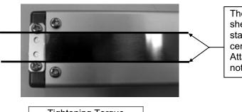
There are two grooves for stainless steel sheet attachment guides. Align so that the stainless steel sheet is positioned at the center between the two grooves. Attach the stainless steel sheet so that it is not bent.
