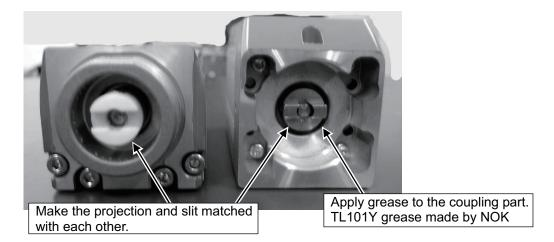
4) Attach the motor unit for replacement with the projection being matched with the slit.
