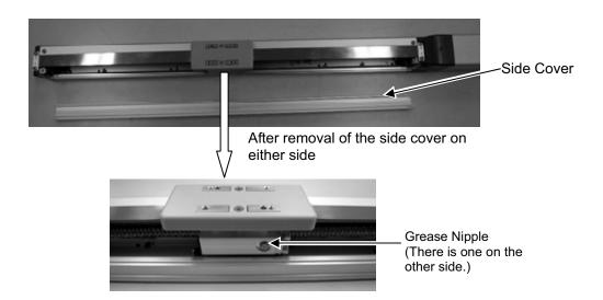
Grease Nipple Diameter [mm] \$\phi 3.5\$
