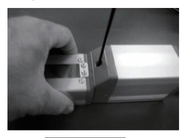
Tightening Torque 353N•cm
