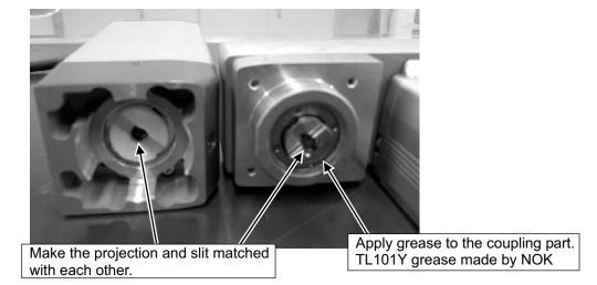
4) Attach the motor unit for replacement with the projection being matched with the slit.
