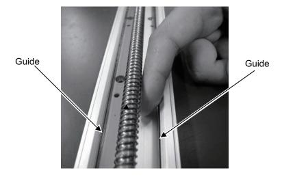
(4) After cleaning up the ball screw, apply the grease with hand. Move the rod back and forth to evenly apply the grease. For some of the low lead actuators, the rod would not move manually with hand. Move it with JOG operation of the controller. Wipe off the excess grease at last.
