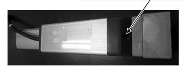
Tightening Torque: 350 N • cm
