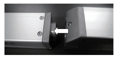
5) Tighten the fixing screw to affixing the motor unit to the actuator with 3mm hex wrench.
