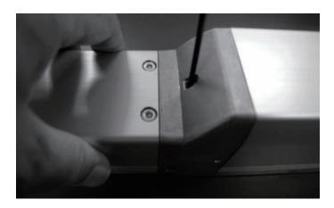
Tightening Torque : 350 N • cm
