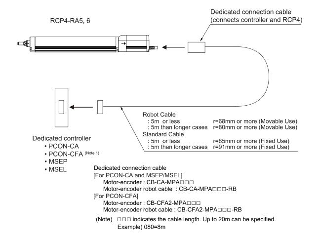
Note 1 Only the motor type 56SP is applicable for PCON-CFA Controller.
