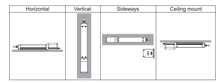
Caution: When the unit is installed vertically oriented, Motor straight type is attempt to put the motor up unless there is a special reason. Putting the motor on the lower side would not cause a problem in an ordinary operation. However, it may rarely cause a problem, when it is not operated for a long period, depending on the surrounding environment (especially high temperature), caused by the grease being separated and the base oil flowing into the motor unit.
