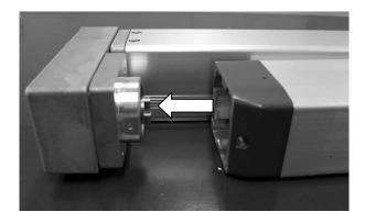
5) Tighten the fixing screw to affixing the motor unit to the actuator with 3mm hex wrench.
