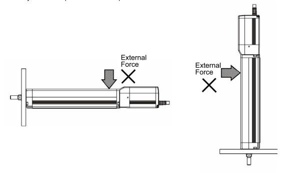
Prepare a support block as shown in the figure below for the horizontal installation of the unit with its stroke more than 150 even if there is no external force applied on the body. Even for those with the stroke less than 150, it is recommended to have a support block to avoid vibration being generated due to the operation condition or installation environment, which may cause an operation failure or parts malfunction.
