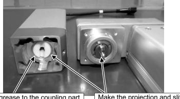
Apply grease to the coupling part. TL101Y grease made by NOK
