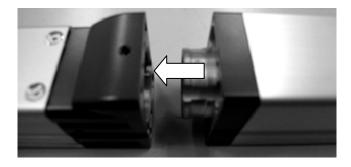
5) Tighten the fixing screw to affixing the motor unit to the actuator with 2mm (RA3C) hex wrench.
