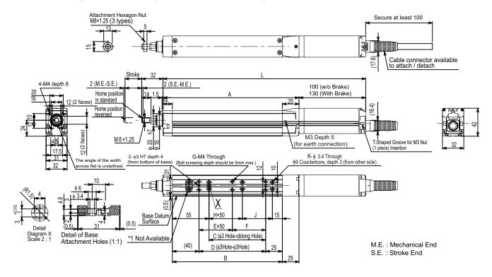
\*1 Two attachment holes on the rod side of the top of the base cannot be used.
