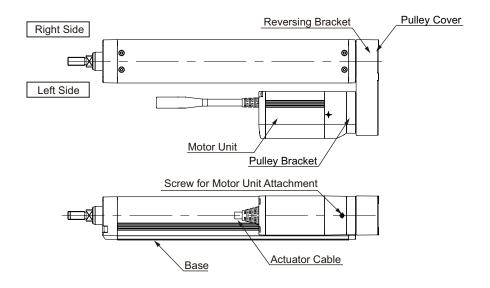
The direction of the motor is either left reversed: ML (shown in figure above) or right reversed: MR.
