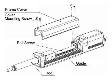
(2) Pull out the rod. The ball screw will appear. For some of the low lead actuators, the rod would not move manually with hand. Move it with JOG operation of the controller.
