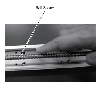
Caution: Supplying too much grease may increase sliding resistance and load to the motor, resulting in a drop of performance.
