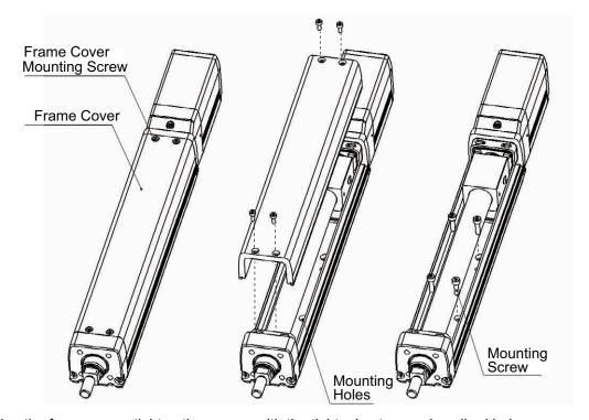
When affixing the frame cover, tighten the screws with the tightening torque described below.
