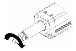
Should be below allowable torque
