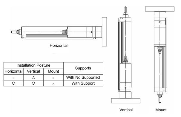
When using the unit in the horizontal or vertical orientation, have a pedestal to support the body to avoid external force being applied to the unit.
