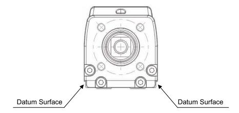
Follow the diagram below when installing the device using the reference surface.
