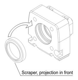
4) Affix the front bracket temporarily. To tune the center of the front bracket, pull out the rod as much as possible and tighten the screws to hold the front bracket.
