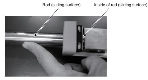
If the unit is equipped with the scraper (optional), apply the grease on the rod sliding surface inside the main unit.
