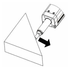
Be careful on the direction of the reaction force against the pressing operation.
