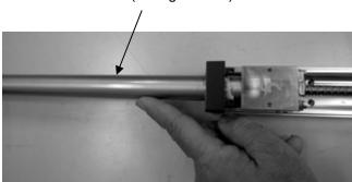
(4) After supplying the grease, attach the frame cover.
