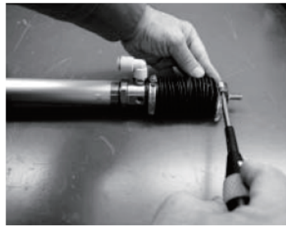
Tightening of front metal fitting
