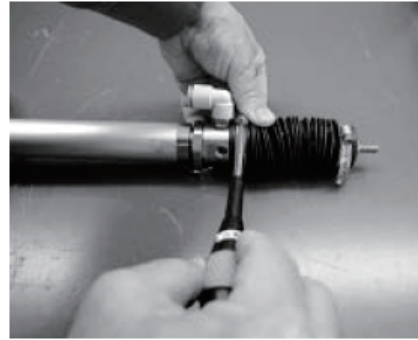
Loosening of rear metal fitting
