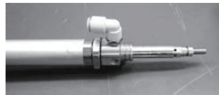
Bellows has been removed
