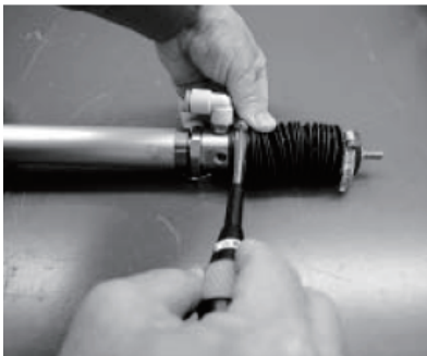
Tightening of rear metal fitting
