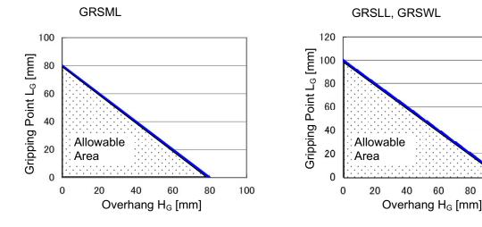
Upper Limit for Gripping Point L<sub>G</sub> and Overhang H<sub>G</sub>
