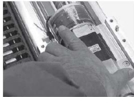
Move the slider. If the actuator is equipped with a brake, release the brake.
