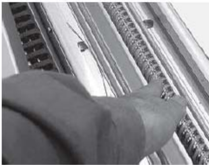
Apply grease on the ball screw.
