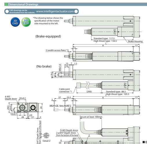
D-M3 Depth 4mm 2-ø3H7 Depth 3mm (from the bottom of the base)
