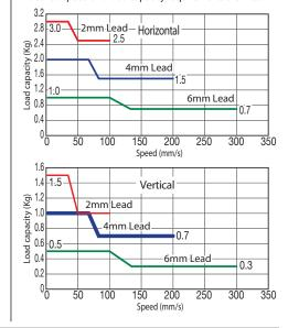
(1) The payload is the value when operated with acceleration of 0.3G (or 0.2G in the case of Lead 2 and vertical usage). The upper limit for acceleration is 0.3G (or 0.2G in the case of Lead 2 and vertical usage).
