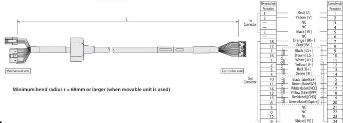
[RCP2 small rotary]-[PMEC] Motor encoder integrated cable for indirect connection
