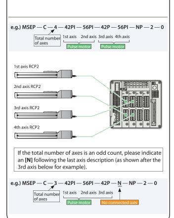
Each board is designed to connect to a pair of axes, and two different types of motors cannot be connected to the same board. Please indicate the same types of motors for each pair of axes.
