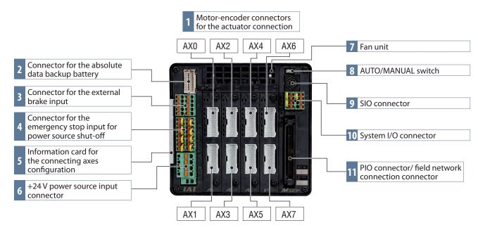
(Note) All the connectors are represented as AX0 through AX7. Please be aware that the motor-encoder cable for the first axis is to be connected to AX0 and the second axis to AX1 respectively.
