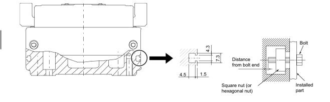
Caution: Square nuts are recommended for use with T-slots, but general hexagonal nuts can also be used. When installing blots in T-slots, pay attention to the length of each bolt to prevent the bolt end from contacting the bottom of the T-slot.
