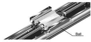
There is no longer metal noise generated by colliding balls and thus noise is reduced. Since balls are aligned by retainers, annoying noise decreases. Wear caused by friction between balls decreases, oil no longer runs out due to contact, and lubricating oil collects at the retainers. Accordingly, operation becomes smooth.
