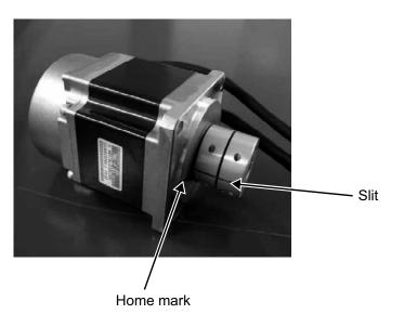
Caution: The motor actuator cable exit direction varies depending on the actuator cable exit direction. The cable exit direction must be the same for the motor to be removed and replacement motor to be installed.
