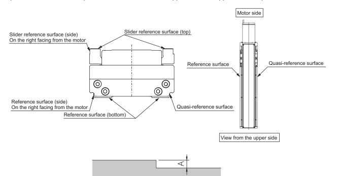
Shoulder dimensions to the base and slider reference surfaces (side)
