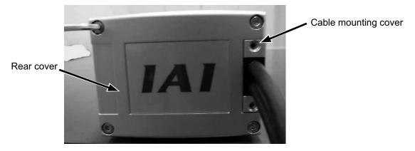
[3] Tighten the screws with an Allen wrench of 2 mm across flats to attach the screws for the cable mounting cover.
