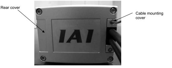
[2] Remove the four bolts used to secure the rear cover using an Allen wrench of 2.5 mm across flats for ISB and ISPB-SXM/SXL, or 3 mm across flats for all other models.
