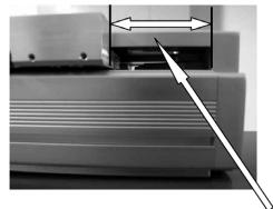
Set this part based on Attachment 2 on Page 84. The use of a block gauge is recommended also in this case.
