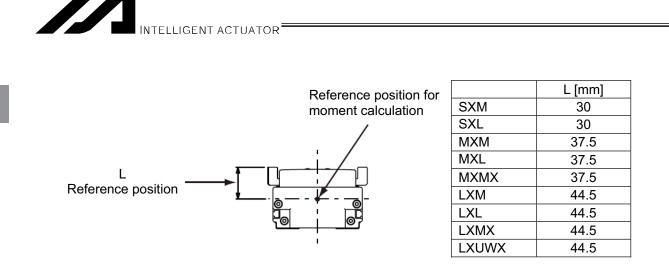
Caution: Make sure the load installed on the actuator is not longer than the allowable overhang load length (L). If the load is longer than L, vibration may occur or the settling time may increase depending on the position of center of gravity position or weight of the work part. If a moment exceeding the allowable moment is applied, not only the life of the guide will become shorter but vibration or longer settling time may also result.
