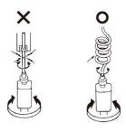
• Do not pinch, drop a heavy object onto or cut the cable
