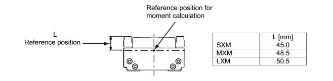
/ Caution: Make sure the load installed on the actuator is not longer than the allowable overhang load length (L). If the load is longer than L, vibration may occur or the settling time may increase depending on the position of center of gravity position or weight of the work part. If a moment exceeding the allowable moment is applied, not only the life of the guide will become shorter but vibration or longer settling time may also result.
