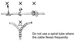
• Separate the I/O and communication lines from the power and drive lines. Do not wire them together in the same duct.
