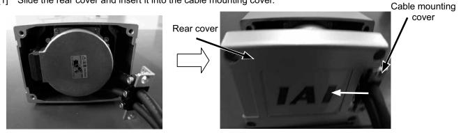
[2] Tighten the four bolts to install the rear cover using an Allen wrench of 2.5 mm across flats for ISB and ISPB-SXM/SXL, or 3 mm across flats for all other models.
