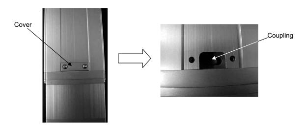
Move the slider to a position where the coupling bolt can be loosened.
