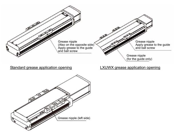
(Note) Follow the grease nipple diameter shown in the list below when preparing a grease gun.
