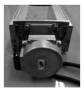
Caution: The cable exit direction must be the same for the motor to be removed and replacement motor to be installed. If the cable exit direction is different on the installed motor, deviation of the home position will
