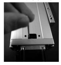
Caution: If the actuator is installed vertically, exercise due caution not to let the slider drop. Hold the slider (work part) from the outside to prevent it from dropping, and then loosen the coupling bolt.
