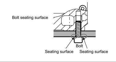
Warning: The threaded holes are not through, so exercise caution when selecting the bolt length. Use of inappropriate bolts may damage the threaded holes or result in insufficient mounting strength of the actuator, leading to a lower precision or unexpected accident.
