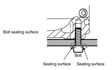
Warning: The threaded holes are not through, so exercise caution when selecting the bolt length. Use of inappropriate bolts may damage the threaded holes or result in insufficient mounting strength of the actuator, leading to a lower precision or unexpected accident.
