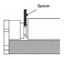
[If a slider jig, etc. cannot be removed] (Note) Apply this method for SSPA since the spacer cannot be put.
