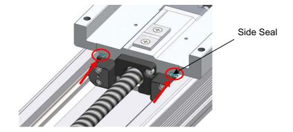
[3] Apply the grease on the ball screw with hand after cleaning it, and move the slider back and forth to spread the grease.
