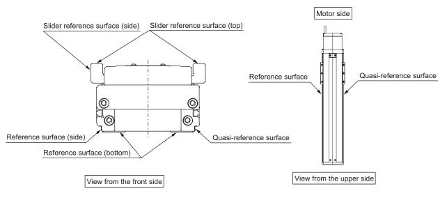
• When using the base or slider reference surface (side), provide a contact surface of the following dimension.
