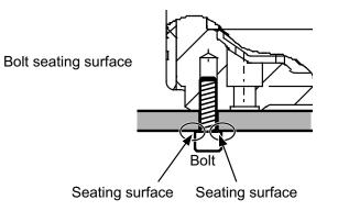
Warning: The threaded holes are not through, so exercise caution when selecting the bolt length. Use of inappropriate bolts may damage the threaded holes or result in insufficient mounting strength of the actuator, leading to a lower precision or unexpected accident.
