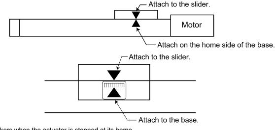
Attach two stickers when the actuator is stopped at its home.
