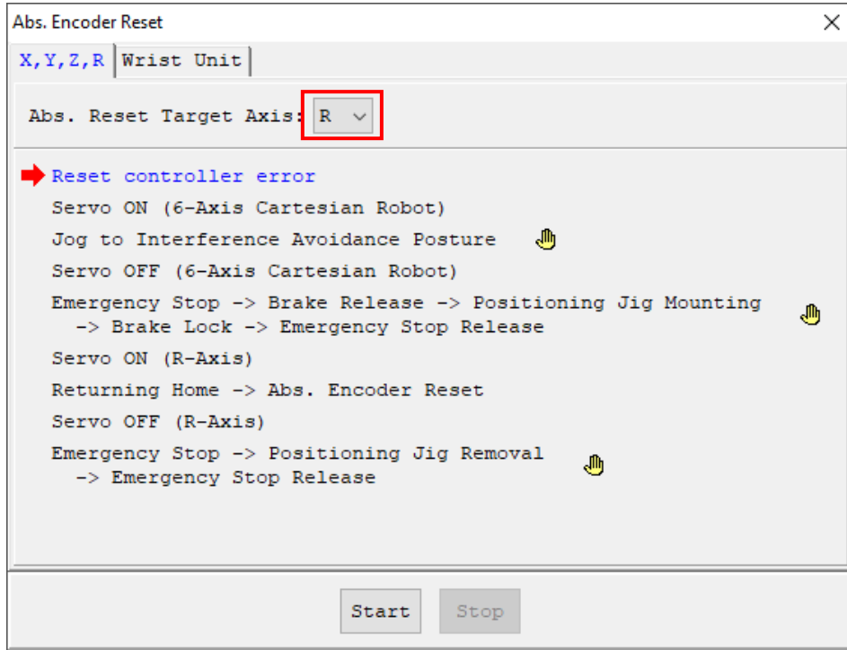
Figure 8.3-6 Abs. Encoder Reset window (6-axis Cartesian Robot)
