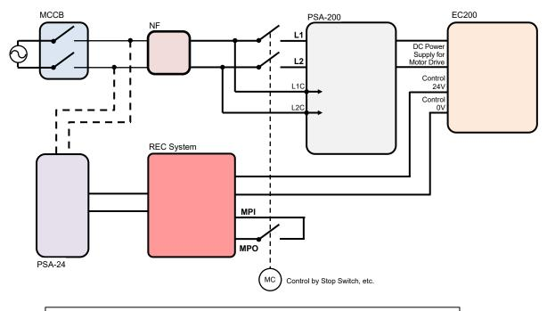
Schematic Diagram for Drive Cutoff of Large Slider Type ELECYLINDER
