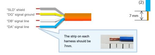
(3) Insert the stripped wiring in the shown in the figure below to the back of the connector and tighten with a flathead screwdriver.
