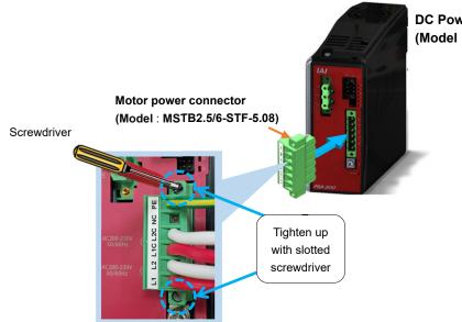
DC Power Supply for Motor Drive (Model : PSA-200-\*)
