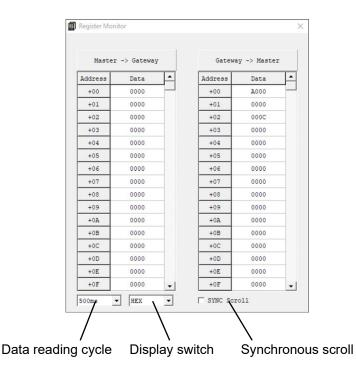
The data that the gateway received from the master and transmission data returned to the master are displayed on this register monitor screen.
