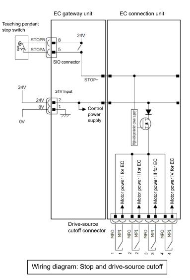
Note 1 When there is nothing to be connected to the SIO connector, STOPA and STOPB should make short-circuit inside the controller.
