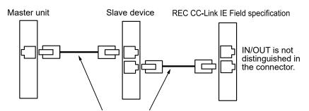
Ethernet straight cable, Category 5e or higher Aluminum tape and braided double cutoff shielded cable recommended (Note) Terminal resistor is not required.
