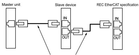
Ethernet straight cable, Category 5 or higher Aluminum tape and braided double cutoff shielded cable recommended (Note) Terminal resistor is not required.
