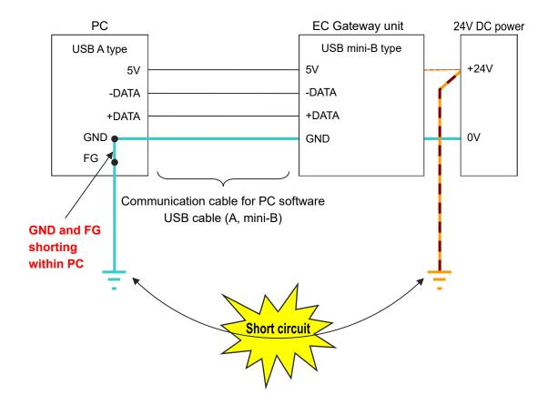
If the EC gateway unit is grounded at the positive terminal of the 24V DC power supply, use an SIO isolator (RCB-ISL-SIO) as shown in the diagram below when connecting a PC to the SIO connector of the EC gateway unit.
