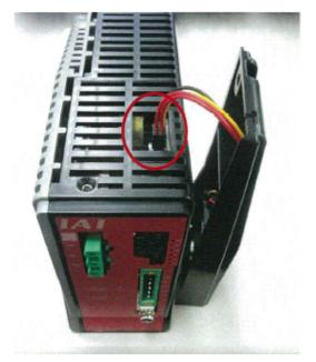
(3) Connect the black connector on the replacement fan unit to the connector on the top of the power supply.
