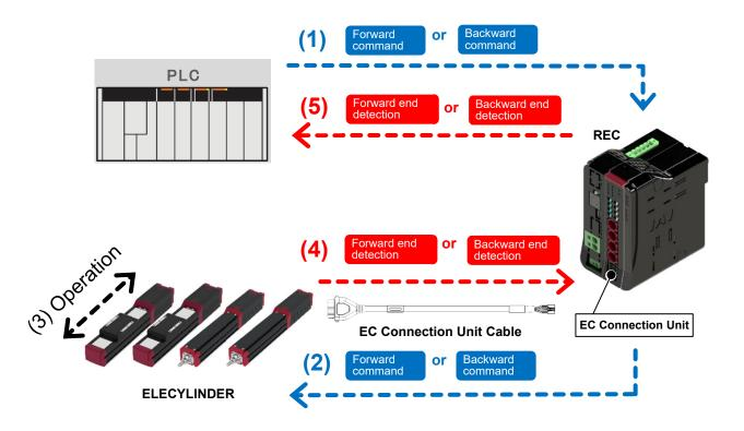
ELECYLINDER continues its operation while a movement command signal (ST0/ST1) is on, and a position detection signal (LS0/LS1) turns on after the operation is complete.
