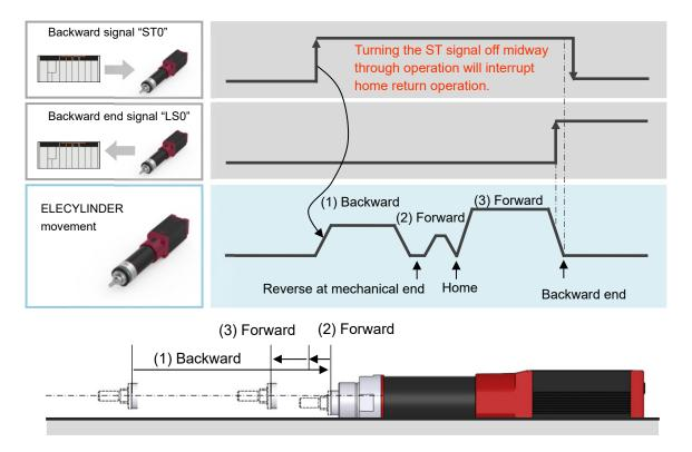
(1) When the "ST0" signal is turned on, backward motion begins towards the mechanical end.
