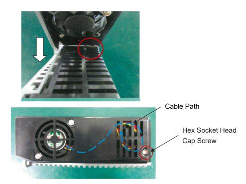
(Note) Pay attention to the cable not to stick it out to the front of the slit on the fan unit.
