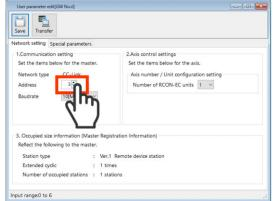
Input a number on the PC keyboard and press the Enter key. The number can also be set with button operation if there is a spin box (small up and down buttons with triangle marks (▲/▼)).
