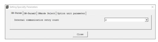
• Internal communication retry count : In AUTO, this is used to set the number of communication retries with the connected axis.
