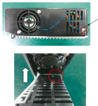
(1) Remove the hex socket head cap screw and take off the fan unit.
