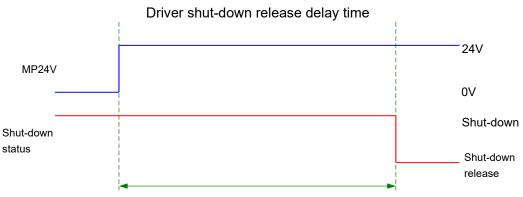
(Driver shut-down release delay parameter) x (Driver number)
