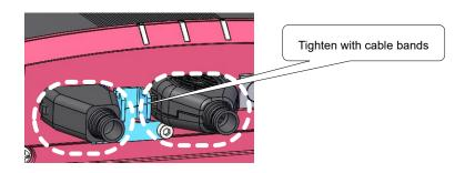
When pulling out the connector, insert a thin tool in a gap between the connector guard and the connector to hold the locking feature, hold the other side at the same time and then pull it out.
