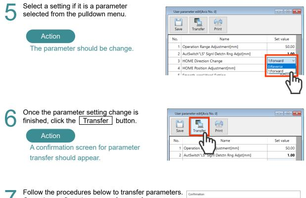
Follow the procedures below to transfer param Once the confirmation screen for transfer to the controller appears, click OK.
