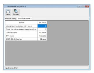
The switchover of the parameter setting screen can be done by clicking "Network setting" and "Special prameters" tags.
