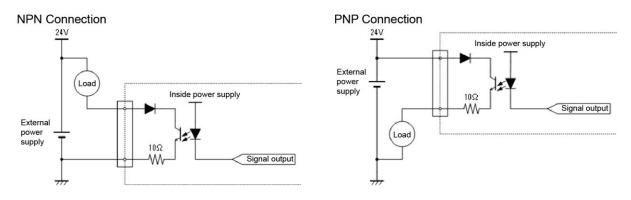
\* In case the current exceeding the maximum load current flows, the circuit may get damaged and the output should become open.
