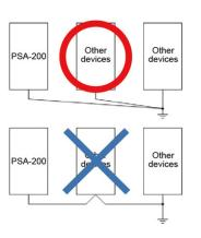
Do not attempt to have the ground line in common with other devices or link it to another. Have it grounded for each power supply unit.
