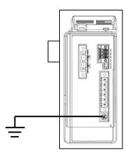
Class D grounding construction (Old Class 3 Grounding: Grounding resistance  $100\Omega$  or less)
