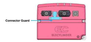
By tightening the matching parts of the connector guard and the connectors with a cable band, concern of contact error at the connectors caused by vibration on the cables can be reduced.
