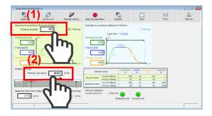
Input a number, press Enter key on your PC keyboard and click Transfer. The number should be written to the controller and Backward end and Forward end buttons turns into green.
