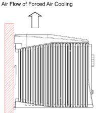
Installing Orientation in Control Panel
