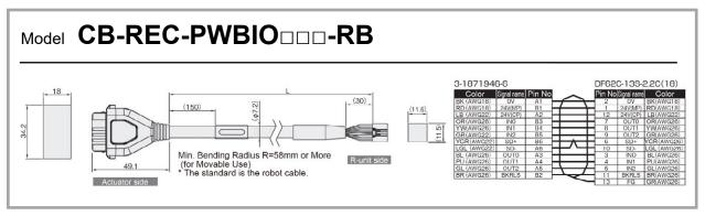
[2] Power Supply / I/O Cable (RCON-EC connection type , 4-way Connector)
