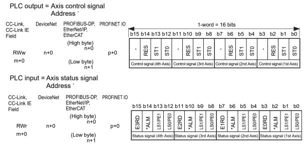
\* m is the head register address of each unit. n is the head relative address of each unit. p is the head module address of each unit.
