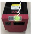
All of maintenance warning LEDs from 1 to 3 on ELECYLINDER flash in green and red in turns.
