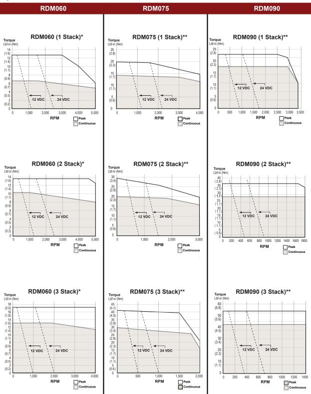
For RDG gearmotors, multiply torque by ratio and efficiency. Divide speed by gear ratio.
