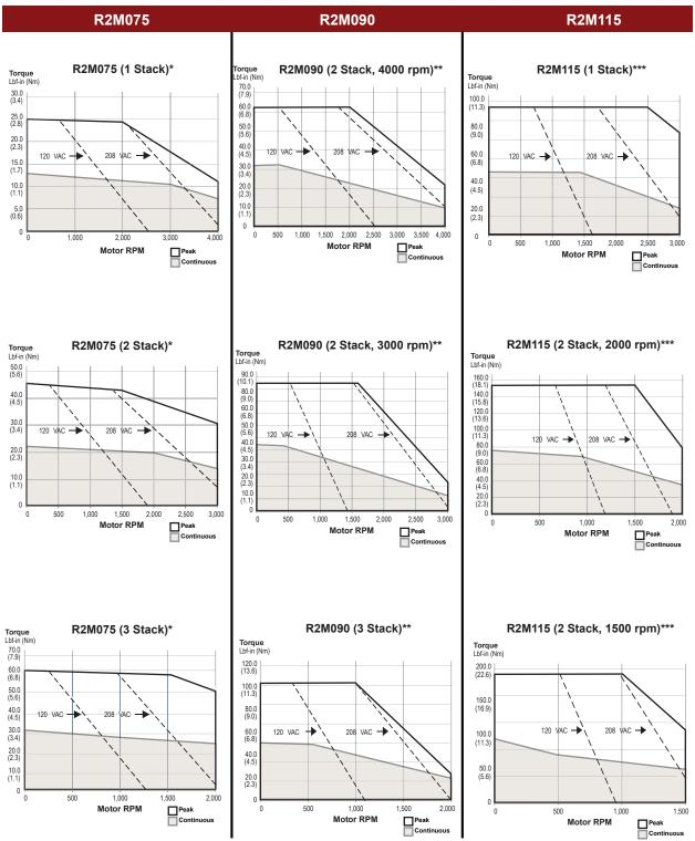
For R2G gearmotors, multiply torque by gear ratio and efficiency. Efficiencies: Divide speed by gear ratio; 1 Stage = 0.91, 2 Stage = 0.86 \*R2M075 test data derived using NEMA recommended aluminum heatsink 10" x 10" x 3/8" at 40°C ambient. \*\*R2M090 test data derived using NEMA recommended aluminum heatsink 10" x 10" x 3/8" at 25°C ambient.
