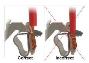
4. Remove the screwdriver. The clamp pressure will keep the wire in place. No exposed wire should protrude past the cage opening
