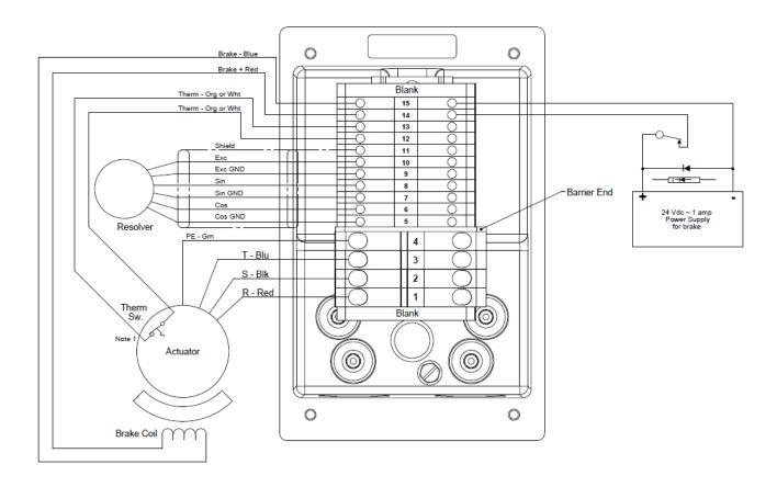
Note 1: Thermal switch normally closed; opens when stator temp exceeds 130 deg. C.
