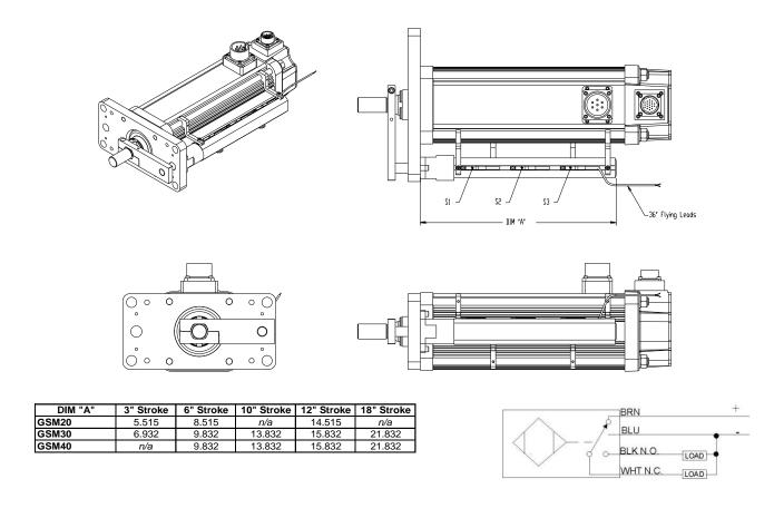
The number of switches desired is selected by ordering the L1, L2 or L3 option, in which 1, 2, or 3 switches will be provided, respectively.
