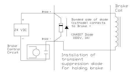
If the user is uncertain about the requirements for transient suppression, they should refer to their servo amplifier or controller technical documentation, or contact their servo amplifier or controller manufacturer for technical support.
