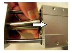
(8) Replenish the grease on the screw shaft. [Refer to 8.5 "Greasing method"]
