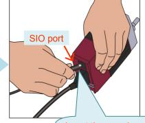
Insert the round connector with arrow mark downward
