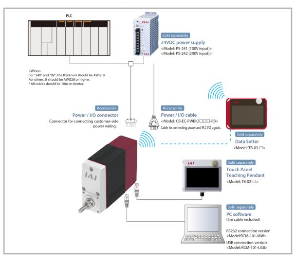
Supply 24VDC to the ELECYLINDER and input a signal from a master device to the ELECYLINDER.
