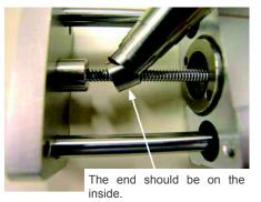
(5) Rolling slightly, press the end onto the shaft end side.
