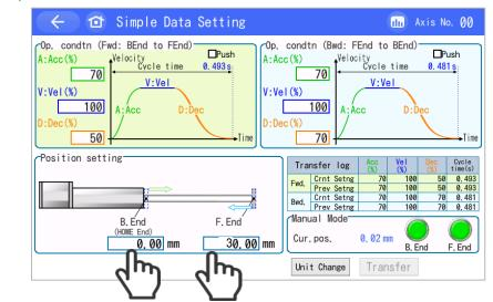
After setting the numerical value, touch the [ENT] key. Then touch the [Transfer] key.
