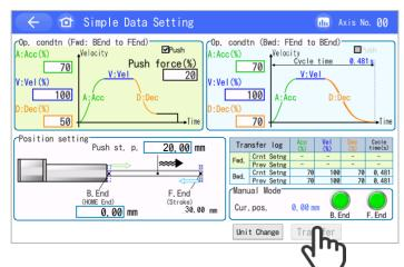
Press the [FEnd] or [BEnd] buttons to operate. Check the results of the new setting/adjustment.
