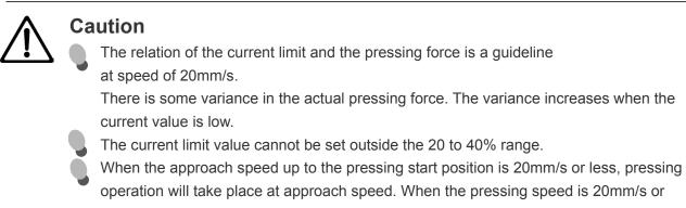
operation will take place at approach speed. When the pressing speed is 20mm/ less, the pressing force will become unstable, and failure to operate normally is possible.
