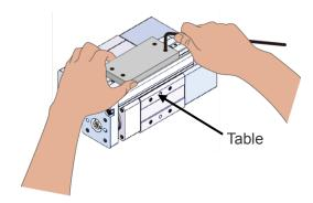
Fixing to both the table top surface and the front plate, which are perpendicular to one another, will affect the rod shaft center and lead to malfunctions.
