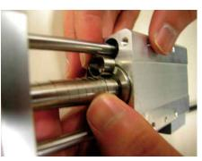
(7) Finally, bring the end to the outside and fit it into the actuator groove.
