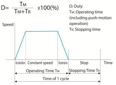
Continuous operation is possible when the duty ratio is 100%.
