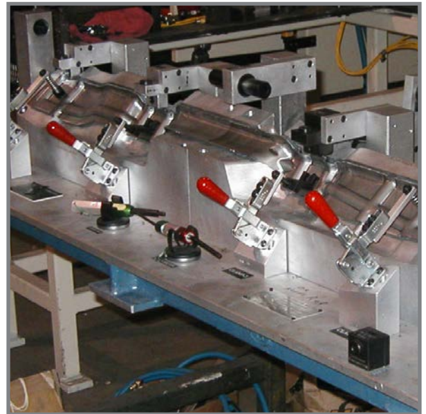
Model 210-U shown being used in a checking fixture application.
