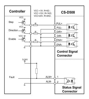
Figure 4: Connections to PNP signal
