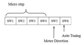
Figure 6: DIP switch Setting
