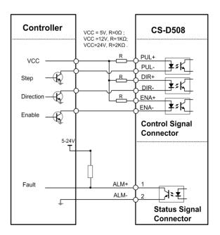
Figure 5: Connections to open-collector signal
