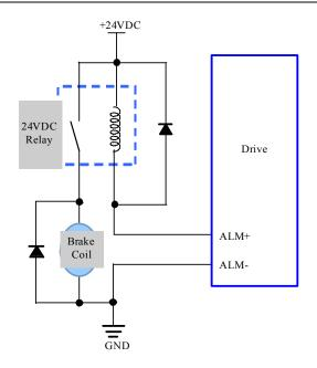
Figure 3: Brake Output Connection
