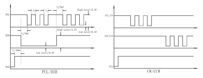
Figure 8: Sequence chart of control signals
