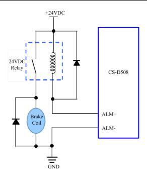
Figure 3: Brake Output Connection
