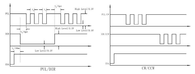
Figure 8: Sequence chart of control signals
