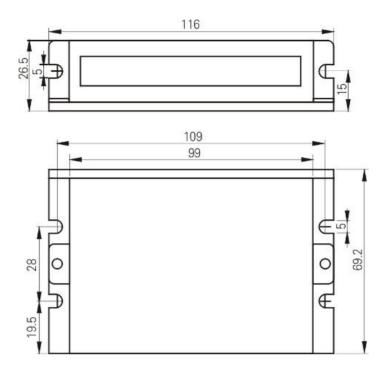
Figure 1: Mechanical specifications
