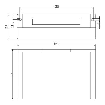
Figure 1: Mechanical specifications
