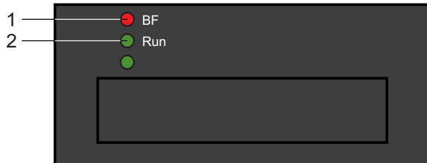
Fig. 36: LEDs for the PROFINET state
