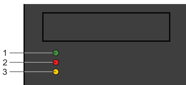
Fig. 33: Diagnostic LEDs on the front of the PS6 device
