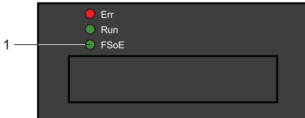
Fig. 37: LED for the FSoE state
